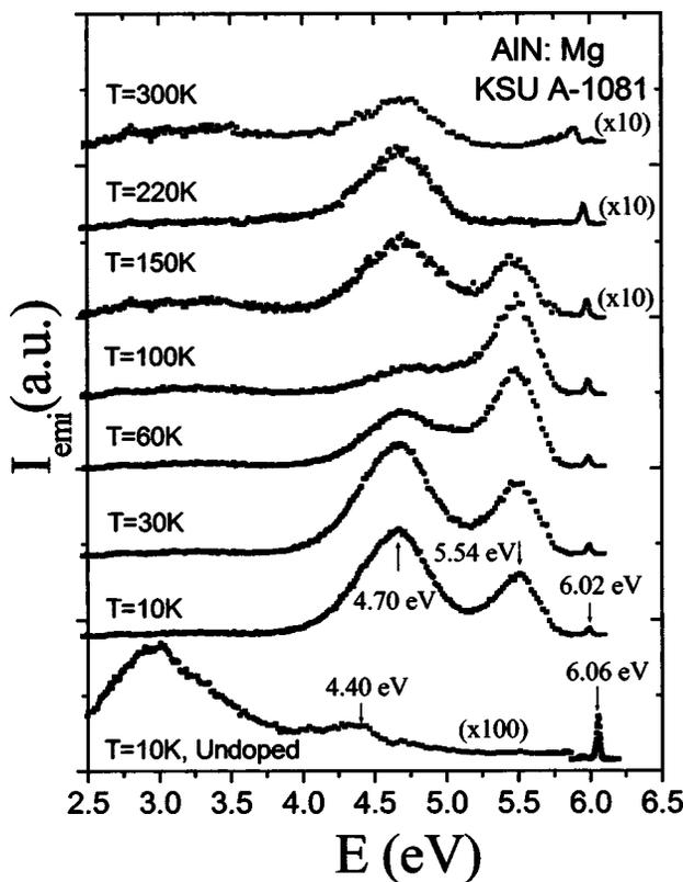
FIG. 1. PL spectra measured at different temperatures for Mg-doped AlN epilayers. The low temperature (10 K) spectrum of an undoped AlN epilayer is also included for comparison.
