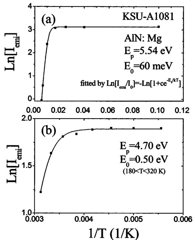
FIG. 2. The Arrhenius plots [ $\ln(I_{em})$ ] vs  $1/T$ ] for two emission lines in Mg-doped AlN: (a) 4.70 eV at  $T < 150$  K and (b) 5.54 eV at  $T > 150$  K. The solid lines are the least squares fits of data with Eq. (1). The fitted activation energies ( $E_0$ ) are indicated in the figure.
