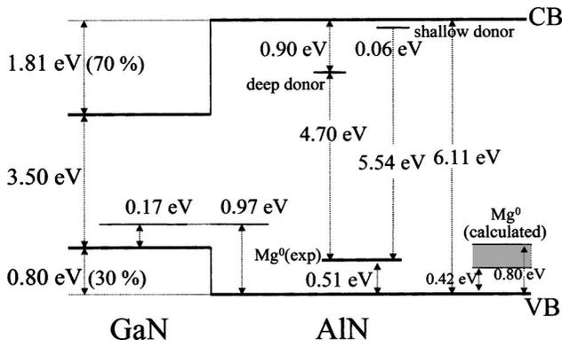
FIG. 3. Energy diagram showing the impurity levels, including Mg acceptor level, in AlN. The upper limit of Mg acceptor level in AlN is estimated to be about 0.97 eV by lining up its energy levels within the band gaps of GaN and AlN near the interface of an AlN/GaN heterojunction. The shaded region shows  $E_A$  predicted by the effective mass theory.
