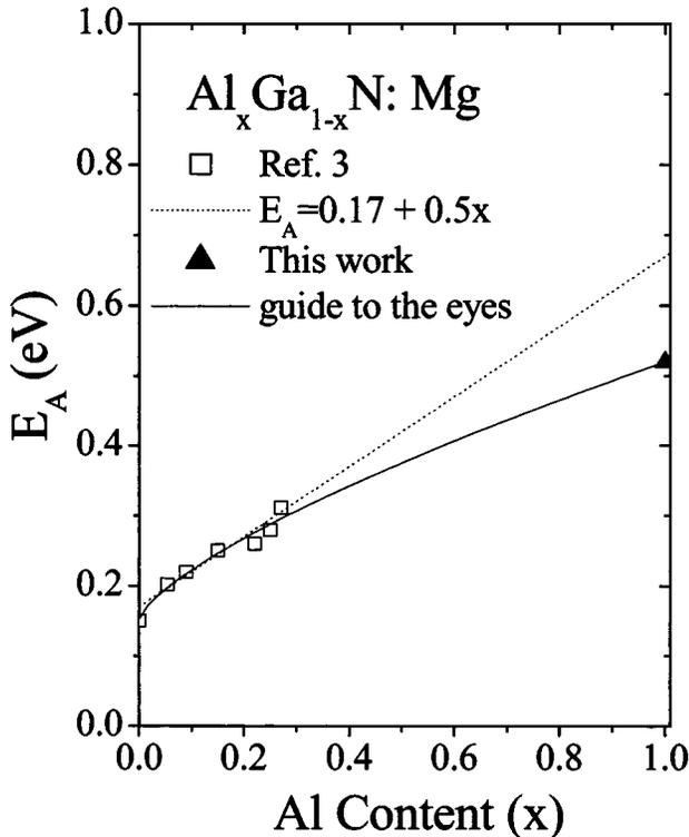
FIG. 4. Mg acceptor activation energy in Mg-doped  $Al_xGa_{1-x}N$  as a function of the Al content ( $x$ ). Closed squares are data from Ref. 3 and references therein, while the filled triangle is the data for AlN of this work. The dotted line is the linear extrapolation of data from Ref. 3 to  $x=1$  and the solid line is a guide to the eyes.
